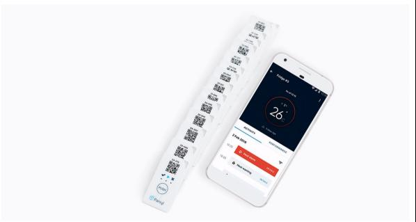
An example of a Parsy data logger used to monitor and capture valuable information about the temperature and humidity commodities are exposed to during transportation and storage.
